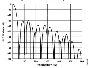
Figure 61. 20 SPS ODR, 50 ms Settling Time
