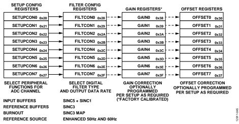
Figure 46. ADC Setup Register Grouping
