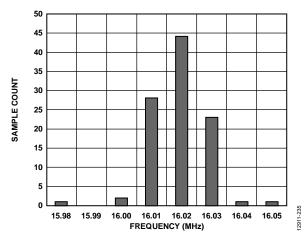
Figure 27. Internal Oscillator Frequency/Accuracy Distribution Histogram (100 Units)
