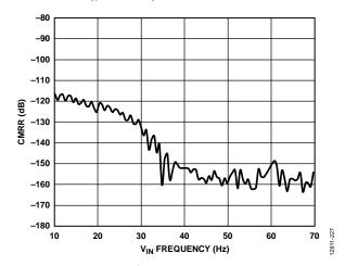
Figure 21. Common-Mode Rejection Ratio (CMRR) vs.  $V_{\rm IN}$  Frequency ( $V_{\rm IN}$  = 0.1 V, 10 Hz to 70 Hz, Output Data Rate = 20 SPS, Enhanced Filter)
