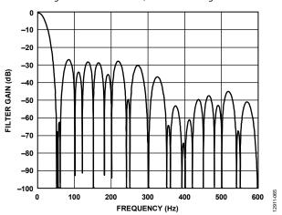
Figure 60. 25 SPS ODR, 40 ms Settling Time
