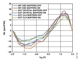
Figure 25. Integral Nonlinearity (INL) vs.  $V_{IN}$  (Differential Input, Internal 2.5 V Reference)
