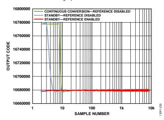
Figure 19. Internal Reference Settling Time
