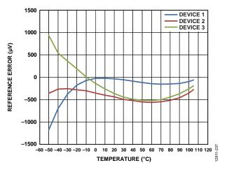
Figure 29. Absolute Reference Error vs. Temperature
