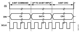
Figure 70. SPI Write Transaction with CRC
