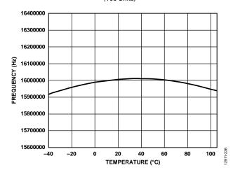
Figure 28. Internal Oscillator Frequency vs. Temperature
