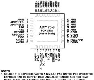
DISSIPATION. THE EXPOSED PAD MUST BE CONNECTED TO AVSS THROUGH THIS PAD ON THE PCB.
