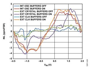
Figure 23. Integral Nonlinearity (INL) vs.  $V_{IN}$  (Differential Input, External 2.5 V Reference)
