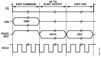
Figure 71. SPI Read Transaction with CRC
