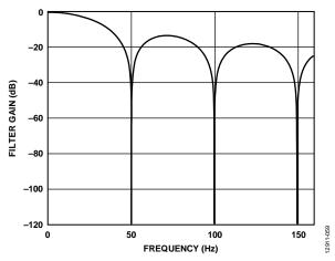
Figure 55. Sinc5 + Sinc1 Filter Response at 50 SPS ODR
