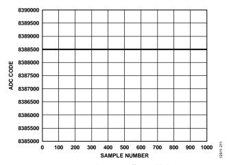
Figure 11. Noise (Analog Input Buffers Enabled,  $V_{REF} = 5 V$ , Output Data Rate = 5 SPS)
