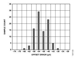
Figure 30. Offset Error Distribution Histogram (Internal Short, 92 Units)
