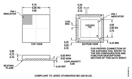
Figure 72. 40-Lead Lead Frame Chip Scale Package [LFCSP\_WQ] 6 mm × 6 mm Body, Very Very Thin Quad (CP-40-14) Dimensions shown in millimeters
