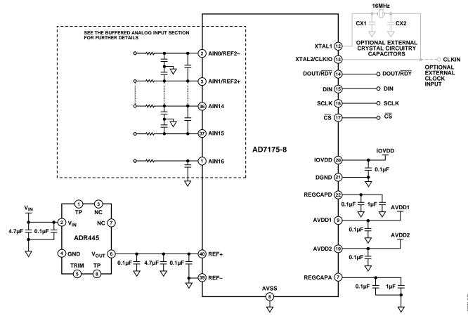
Figure 41. Typical Connection Diagram
