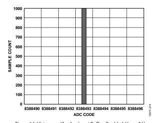
Figure 14. Histogram (Analog Input Buffers Enabled,  $V_{\it REF} = 5$  V, Output Data Rate = 5 SPS)
