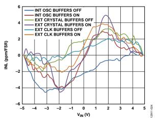
Figure 24. Integral Nonlinearity (INL) vs.  $V_{IN}$  (Differential Input, External 5 V Reference)
