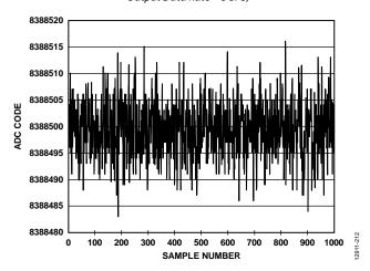
Figure 12. Noise (Analog Input Buffers Enabled,  $V_{REF} = 5 V$ , Output Data Rate =  $10 \, \text{kSPS}$ )
