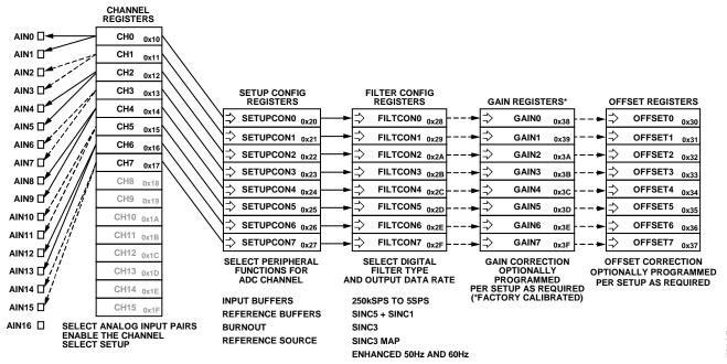
Figure 48. Eight Fully Differential Inputs with a Setup per Channel Rev. 0 | Page 23 of 64
