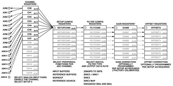
Figure 47. Eight Fully Differential Inputs, All Using a Single Setup (SETUPCONO; FILTCONO; GAINO; OFFSETO)
