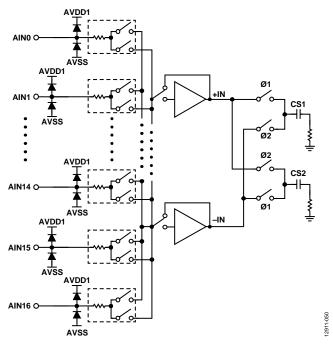
Figure 51. Simplified Analog Input Circuit
