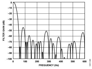
Figure 65. 16.667 SPS ODR, 60 ms Settling Time
