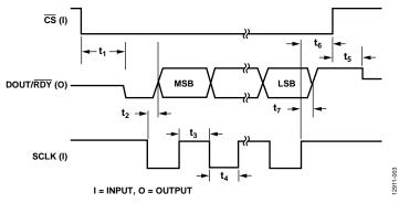
Figure 2. Read Cycle Timing Diagram
