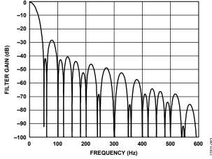
Figure 59. 27.27 SPS ODR, 36.67 ms Settling Time
