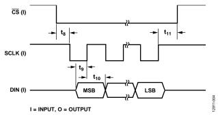
Figure 3. Write Cycle Timing Diagram
