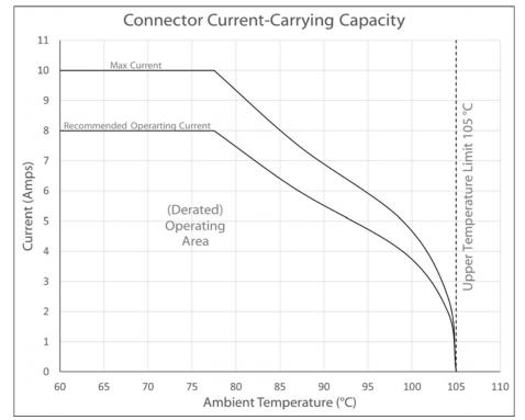
Testing based on IEC 60512-5-2. Max current curve generated with isolated test article under controlled environmental conditions, and does not take into account external factors such as housings or circuitry. Recommended operating current curve accounts for external factors, manufacturing variation, and error in temperature measurements.
