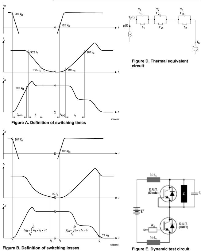
**Figure E. Dynamic test circuit** Leakage inductance  $L_{\sigma}$  =180nH and Stray capacity  $C_{\sigma}$  =180pF.
